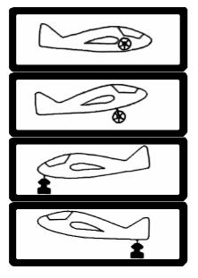
Landing gear up - black handle on the upper left side wall pulled.
